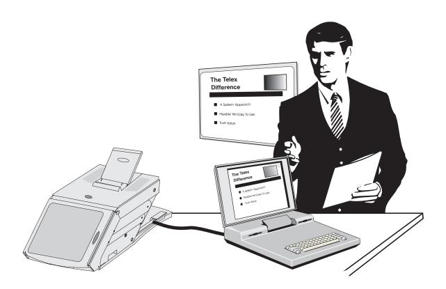
The Firefly<sup>™</sup> P350 can be connected to any IBM or IBM compatible computer equipped with a VGA/SVGA video output. The P350 can also be connected to any Apple Macintosh computer that is equipped with a standard Macintosh video output.
